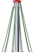
In the centre of the Spire net is the mast, made of high-quality seamless steel. The structure of the mast as an oscillating support which is statically favourable and equalises the oscillations in the Spire Net. The masts are hotdipped galvanised as standard.
