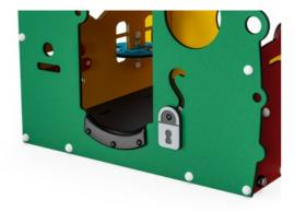
Floor is made of HPL with a thickness 10 mm and non skid surface texture according to EN 438-6. KOMPAN HPL has high wearing strength to ensure long lifetime in all climates.
