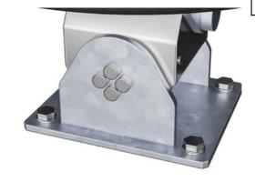
The double ROSTA element is made of ductile iron and has a hot-dip galvanized finish before painting. The ROSTA element is maintenance-free, with a elastic joint capable of a range of motion up to 250 degrees in any direction. Both wobbles have different stiffness, with a 45% disparity.
