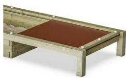
Boards are made of pine wood from sustainable European sources. The wood is pressure impregnated Class 3 with Tanalith E3475 according to EN335 (Equivalent to NTR Class AB).
