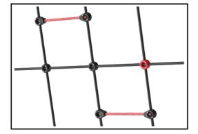
Ropes are made of UV-stabilized PES rope strands with inner steel cable reinforcement. The polyester wrapping is inductively melted onto each strand to ensure excellent wear and tear resistance.
