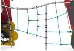
Ropes are made of UV-stabilized PP rope strands with inner steel cable reinforcement. Horizontal ropes are PUR coated to obtain good wear and tear resistance. The steel surfaces are hot dip galvanised inside and outside with lead free zinc. The galvanisation has excellent corrosion resistance in outside environments and requires low maintenance.
