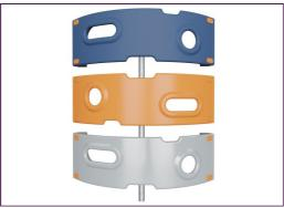
The climbing elements displayed are moulded from 33% post-consumer recycled materials in one piece, with a minimum 5mm wall thickness. The climbing elements are made of recyclable PE which has a high impact resistance across a wide temperature span which ensures vandal resistance in all locations.
