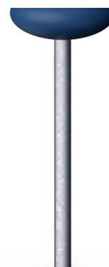
The tube of the Grasshopper is made of a Ø48,3 x 2,9mm, hot dip galvanized steel tube. The top seat is connected with a M12 bolt and covered by a PE top cap.
