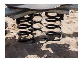
KOMPAN Springs are made of high quality spring steel according to EN10270. The springs are cleaned by phosphating before they are painted with an epoxy primer and a polyester powder coating as top finish. The springs are fixed by unique anti pinch fittings for maximum safety and long lifetime.
