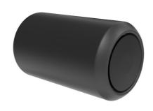
The rotating rollers are Ø 110mm and made from PUR (Polyurethane Rubber, compact foam). The rollers have a steel insert that is electro galvanized. They provide support and ensure a comfortable position.
