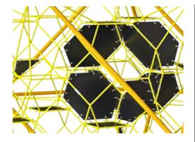
Corocord membranes consist of friction-proof rubberized material of conveyor belt quality with excellent UV resistance. Tested and compliant with REACH requirements for PAH. Embedded is a four-layered armouring made of woven polyester. The armouring and the two surface layers result in a total thickness of 7.5 mm.
