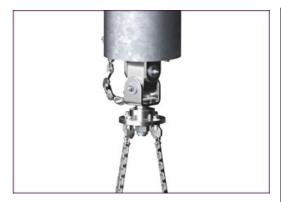
Unique designed 360-degree rotating swing hanger made of stainless steel. The moving parts of the swing hanger is lifetime sealed and lubricated. The hanger system is equipped with a safety chain to prevent the swing hanger to fall down if damaged.
