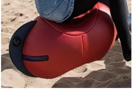
The seat is made with recycable PE from 33% post consumer materials and moulded in one piece with a minimum 5mm wall thickness. PE has high impact resistance across a wide temperature span which ensures vandal resistance in all locations.
