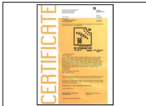
The HDPE sail is authorized to use the UV-label grade 10 in accordance with UV standard 801 under the test report number 738740-1. See certificate on [www.master.KOMPAN.com](http://www.master.KOMPAN.com)
