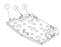
A 5 mm hot-dip galvanised carbon steel plate must is moulded inside the SBR to offer optimal stability and optimize the mounting of the step to the frame.
