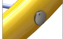
The rope is fixed to the large steel pipe by a unique KOMPAN designed tightening solution. It consists of inner and outer nylon (PA6) bushings that guides the rope to an outside threaded aluminum part that tighten the rope.
