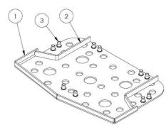
The polyurea coating, used on all grips, is highly A 5 mm hot-dip galvanised carbon steel plate must is moulded inside the SBR to offer optimal durable against wear and tear, offers isolation and simultaneously gives users an outstanding stability and optimise the mounting of the step to the frame.
