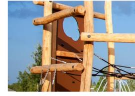
Plywood climbing panel. The climbing panels is made of 21,5mm thick plywood made from alder and pine wood. Both sides are covered by 2 layers of phenolic film with anti slip net pattern. All cutting edges are sealed with paint to ensure long lifetime
