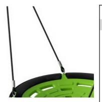
The shell seat is made of 100% recyclable polyethylene (PE) and rotomoulded in one piece. The seat is designed with large outer openings for handholds and middle holes, allowing for drainage of water and dirt. The four ropes are attached with hot-dip galvanised steel brackets to ensure durability for many years.
