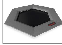
The tiles are molded in grey granulated recycled rubber (SBR/NR), and the KOMPAN logo is made of EPDM Ethylene Propylene Diene Monomer. Inside each of the rubber tiles there is a 3 mm hot dip galvanized steel plate.
