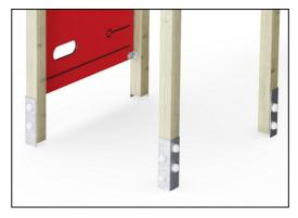
The main posts are equipped with hot-dip galvanised steel footings. The steel footings elevate the posts position 20mm from ground level to avoid contact with surfacing material.
