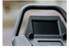
The handle bars are designed with multiple hand positions to accommodate different postures and riding styles. It is a casted Aluminum part with Polyurea coating for good grip and insulation.
