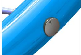
The rope is fixed to the large steel pipe by a unique KOMPAN designed tightening solution. It consists of inner and outer nylon (PA6) bushings that guides the rope to an outside threaded aluminum part that tighten the rope.
