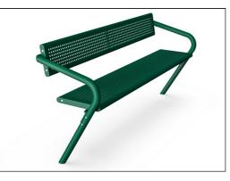
Powder coated top finish on top of galvanization is processed in two steps: Light grinding and clean sweeping, powder coating - thickness 70-120 µm.
