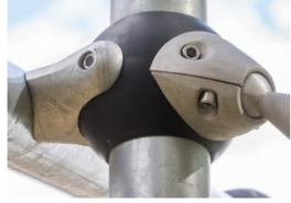
The unique designed GALAXY connection ball is produced with an inner circular core of aluminium surrounded by a shell of hard PP with an outer layer of soft TPV rubber. Flexible lead-free aluminium connectors allow for installation in variable angles.
