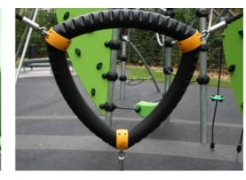
GALAXY climbing triangle with an outer soft layer of PUR and corner brackets of moulded nylon (PA6). The core consists of a powdercoated welded steel frame with integrated corner suspension points. Larger triangles are closed with an 18mm thick Ekogrip® panel that has a top layer of rubber with a non-skid effect.
