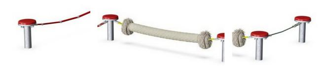
Balance pads are made of EPDM rubber. Material is UV stabalised. The PP rope in coconut style has a diameter of 150 mm. The internal steel wire core has thimbles at both ends, which serve as attachments for the rope to existing connecting elements.
