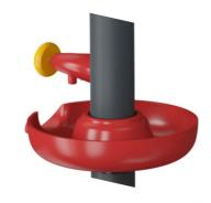
The integrated water tap open for water when pushed and stops when letting go. The water is supplied trough a pipe located inside the post with hose or pipe connection at the bottom of the post. The supply can either a loose hose or a permanent in-ground pluming.
