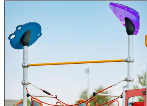
The support frame is  $\varnothing 48.3 \times 4$ mm, carbon steel, with a hot-dip galvanised surface according to ISO1461, and a powder coating corrosion class C3 according to ISO12944-2. Lead content for surfaces is below 90ppm.
