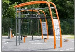
To ensure the integrity of the main frame, the orange coloured main posts are made of ø101.6 x 3mm steel posts, which are hot dip galvanised and powder coated Orange (RAL2010). The supportive posts receive the same surface treatment and are made of ø76.1 x 3.6mm steel tubes, powder coated grey (RAL7012).
