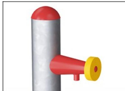
The integrated water tap open for water when pushed and stops when letting go. The water is supplied through a pipe located inside the post with hose or pipe connection at the bottom of the post. The supply can either be a loose hose or a permanent in-ground plumbing.
