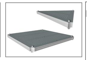
All decks are made of perforated low carbon steel plates supported by aluminum profiles with no unsupported area larger than four square feet. After metallization the decks are coated with a polyurea non-slip surface which provides extremely good wear and tear resistance.
