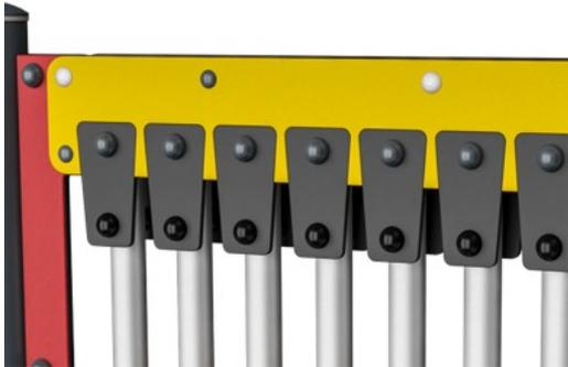
Membranes consist of friction-proof rubberized material of conveyor belt quality with excellent UV resistance. Embedded is a four-layered armoring made of woven polyester. The armoring and the two surface layers result in a total thickness of 9 mm.
