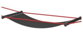
Corocord membranes consist of friction-proof rubberized material of conveyor belt quality with excellent UV resistance. Tested and compliant with REACH requirements for PAH. Embedded is a four-layered armouring made of woven polyester. The armouring and the two surface layers result in a total thickness of 7.5 mm.
