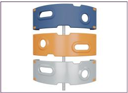
The climbing elements displayed are moulded from 33% post-consumer recycled materials in one piece, with a minimum 5mm wall thickness. The climbing elements are made of recyclable PE which has a high impact resistance across a wide temperature span which ensures vandal resistance in all locations.
