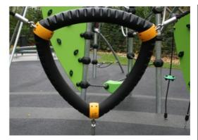
GALAXY climbing triangle with outer soft layer of PUR and corner brackets of moulded nylon (PA6). The core consist of a powder coated welded steel frame with integrated corner suspension points. Larger triangles are closed with an 18mm thick Ekogrip® panel that has a top-layer of rubber with a non-skid effect.
