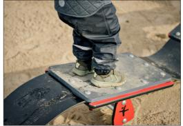
The two central plates on the Wave Stepper are of made of Ekogrip® panels that consist of a 15mm thick PE base with 3 mm top-layer of soft rubber with a non-skid effect.
