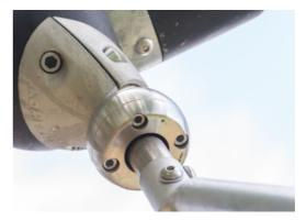
Bearing systems has been designed to be heavy-duty and maintenance free. All steel bearings are fully closed and lifetime lubricated.
