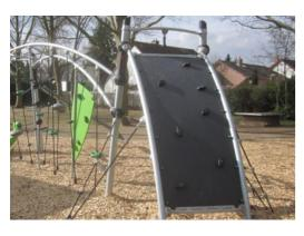
The curved climbing wall is manufactured from a steel frame and an Ekogrip® panel with unique designed climbing cleats. The Ekogrip® panel is constructed from a 5mm thick PE base with 3 mm top-layer of rubber with a non-skid effect.
