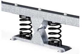
KOMPAN Springs are made of high quality spring steel according to EN10270. The springs are cleaned by phosphating before they are painted with an epoxy primer and a polyester powder coating as top finish. The springs are fixed by unique anti pinch fittings for maximum safety and long lifetime.
