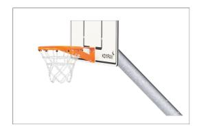
The basketball hoop is made from hot dipped galvanized steel with a powder coated finish. The net is made from Ø4 chain links made from s235 Galvanized steel or stainless-steel chains which meet the requirements in ISO1434-ISO1435 and DIN766. The chains have a circumference of ~Ø30cm at the bottom and ~Ø50cm at the top.
