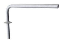
The bar is 1400mm long, with a height of 940mm and is intended as grip during exercises. The bar is made of hot-dip galvanized steel ø38mm, a great diameter for a good grip and to support the wrist.
