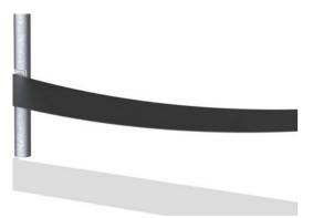
Membrane consisting of friction-proof rubberized material of conveyor belt quality with excellent UV resistance. Tested and compliant with REACH requirements for PAH. Embedded are two layers of galvanised steel wire armoring, making the membrane extremely hardwearing and vandalism resistant. Core and outer layers result in a total thickness of 10mm.
