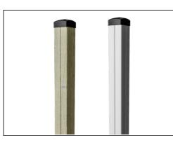
The main tower posts are available in two types of material: European pine wood posts, pressure impregnated Class 3 with Tanalith E3475 according to EN335 (Equivalent to NTR Class AB). Aluminum post t=2mm with anodized surface treatment. Base material EN AW-6060 T66.
