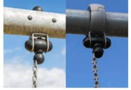
The swing hangers are made of high quality UVstabalized nylon (PA6) housing with integrated lifetime sealed ball bearings. The height adjustable chains are fixed by a stainless steel hook with theft proof snake-eye bolt in a turn able anti twist housing. All seats with two chain fixation are available with either standard or anti-wrap suspension.
