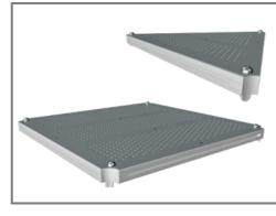
All decks are made of perforated low carbon steel plates supported by aluminum profiles with no unsupported area larger than four square feet. After metallization the decks are coated with a polyurea non-slip surface which provides extremely good wear and tear resistance.
