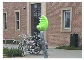
The coloured top is made of injection moulded high quality nylon (PA6) which is UV stabilised to ensure long life time. The two component design is assembled with steel pins around the steel pipe.
