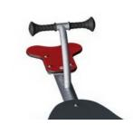
Handles are made with a moulded PP insert and an outer layer of soft TPV rubber. The handles are attached to the pipe with a galvanised steel inlay to ensure strength and durability.
