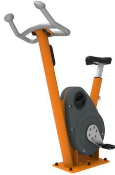
The front tube for the frame is made of S235 hot-dip galvanized steel tubing with the following dimensions  $\varnothing 76,1 \times 3,6$ mm. and with a powder coating corrosion class C3 according to ISO12944-2.
