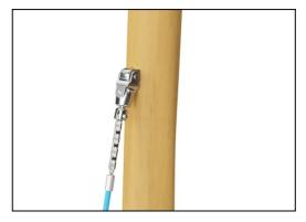
The swing hangers are made of stainless steel brackets and can move over two axis. The flange bearings are silicone enriched to make the suspension maintenance free. The connection to the rope is made with stainless steel chain.
