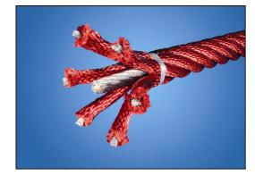
Corocord ropes of UV-stabilized PES rope strands with inner steel cable reinforcement. The polyester yarn is made from +95% post-consumer materials and is inductively melted onto each strand. PES has high strength with excellent resistance to abrasion and UV radiation. The ropes are connected by stainless steel S-Clamps which are pressed around the rope which results in a durable and vandalism solution 12024
