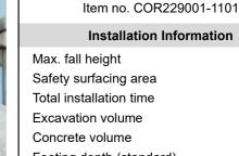
Installation Information 250 cm Safety surfacing area 70.7 m<sup>2</sup> Total installation time 13.6 Excavation volume 10.21 m<sup>3</sup> Concrete volume 6.50 m<sup>3</sup> Footing depth (standard) 110 cm Shipment weight 674 kg Anchoring options In-ground
